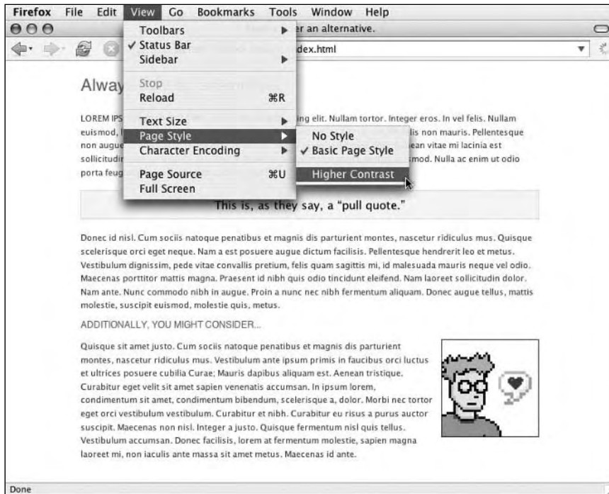
Figure 8-4: By changing the rel attribute of the second link element to “alternate stylesheet” and supplying a title, we’ve implemented some basic style switching.
