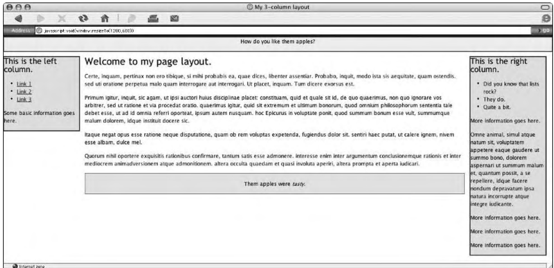
Figure 7-26: In browsers that don't respect the max-width CSS property (such as Internet Explorer on the Mac, shown here), the page layout will simply expand to the width of the window.
