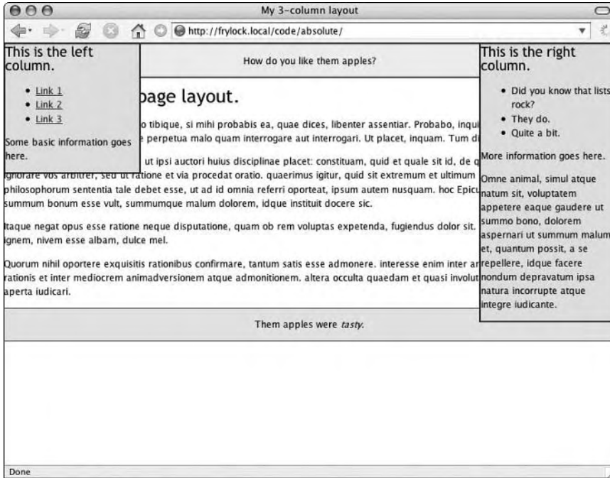
Figure 7-11: Absolute positioning allows us to place the left- and right-hand columns—however, we're not out of the woods yet.
